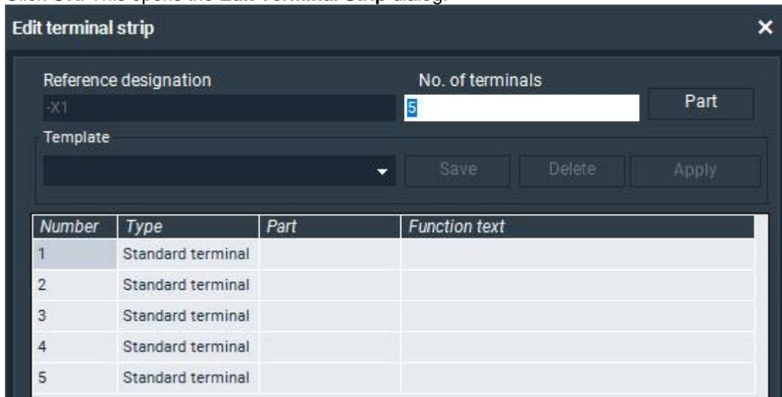
8. Enter the value 5 in the **No. of terminals** field. This creates 5 terminals for the terminal strip.
