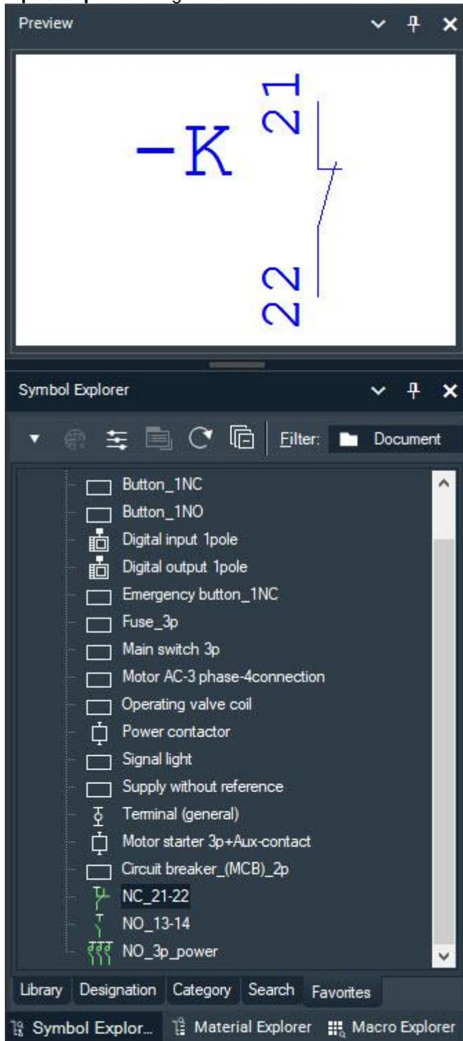
18. Place the auxiliary contact on the line above the spool -Q5.
