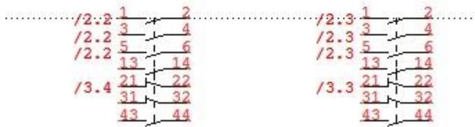
The cross-references to the contacts of the contactor are shown on the left side of the comb.
