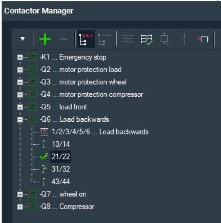
20. Click **OK**. The Contactor Manager is closed. The symbol hangs on the mouse pointer. Cancel the new placement with the right mouse button. The auxiliary contact shows a cross reference to the coil /3.4, drawing sheet 3, path 4).
