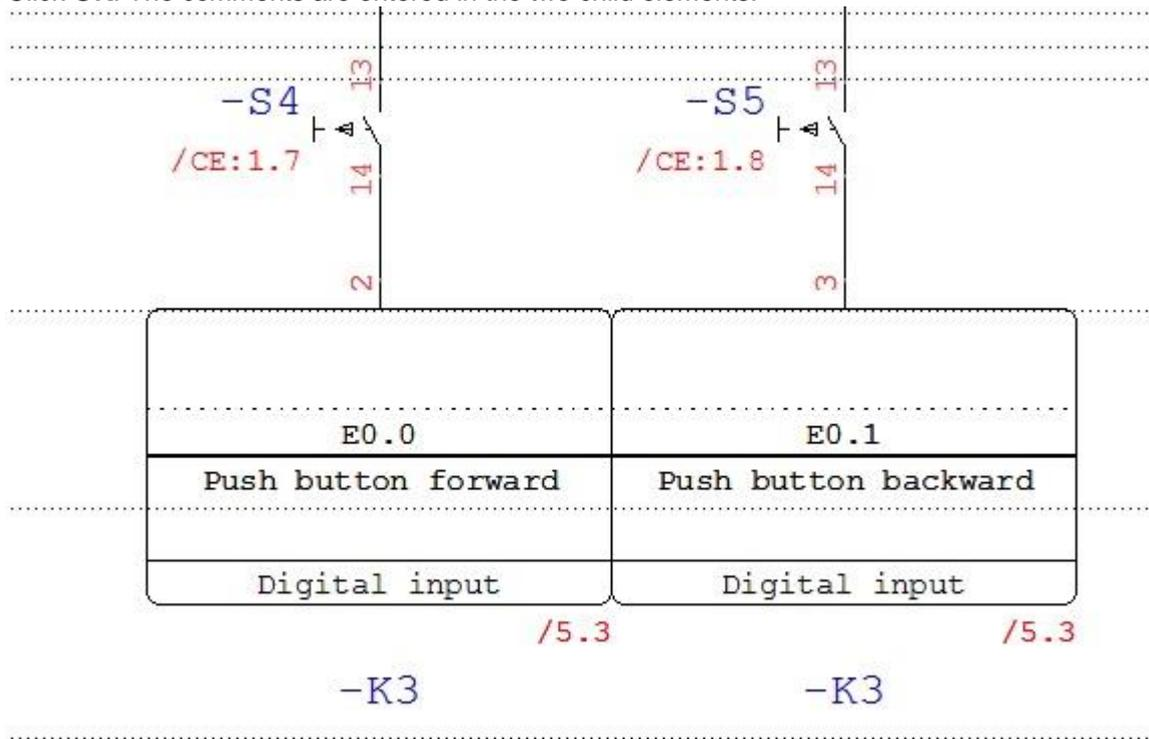
17. Double-click in the Project Explorer on the drawing sheet **Schematics | 0005: PLC chart**. The comments of the two channels are also displayed at the parent element -K3.
