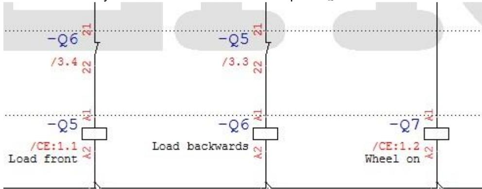
19. The Contactor Manager opens. Click the third sub-item of the contactor -Q6. This defines the auxiliary contact as the normal closer of the contactor -Q6 with the pin number 21/22.
