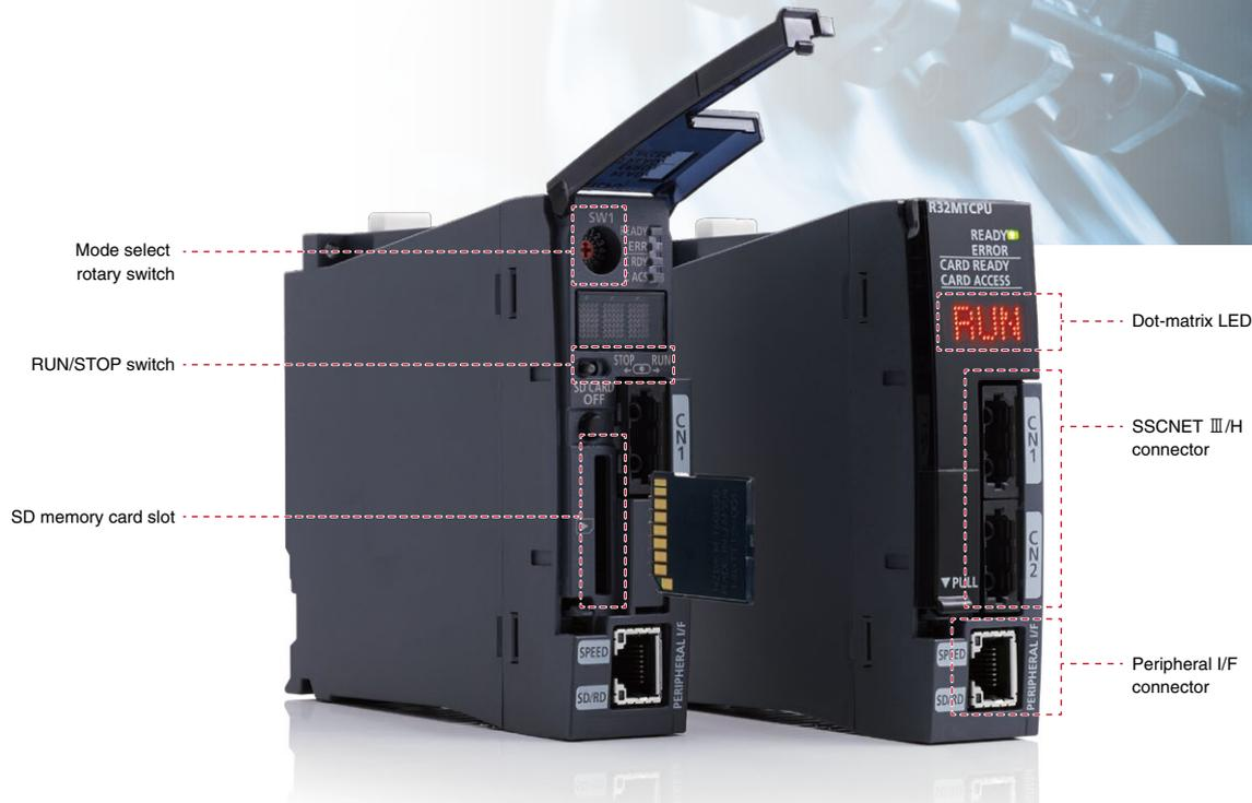
The motion CPU module is a dedicated high-precision control CPU module, designed solely for applications that require advanced motion control such as positioning control, synchronous control, and speed-torque control at a very high accuracy. The motion CPU is incorporated into the multiple CPU architecture of the MELSEC iQ-R Series complementing the programmable controller CPU.
