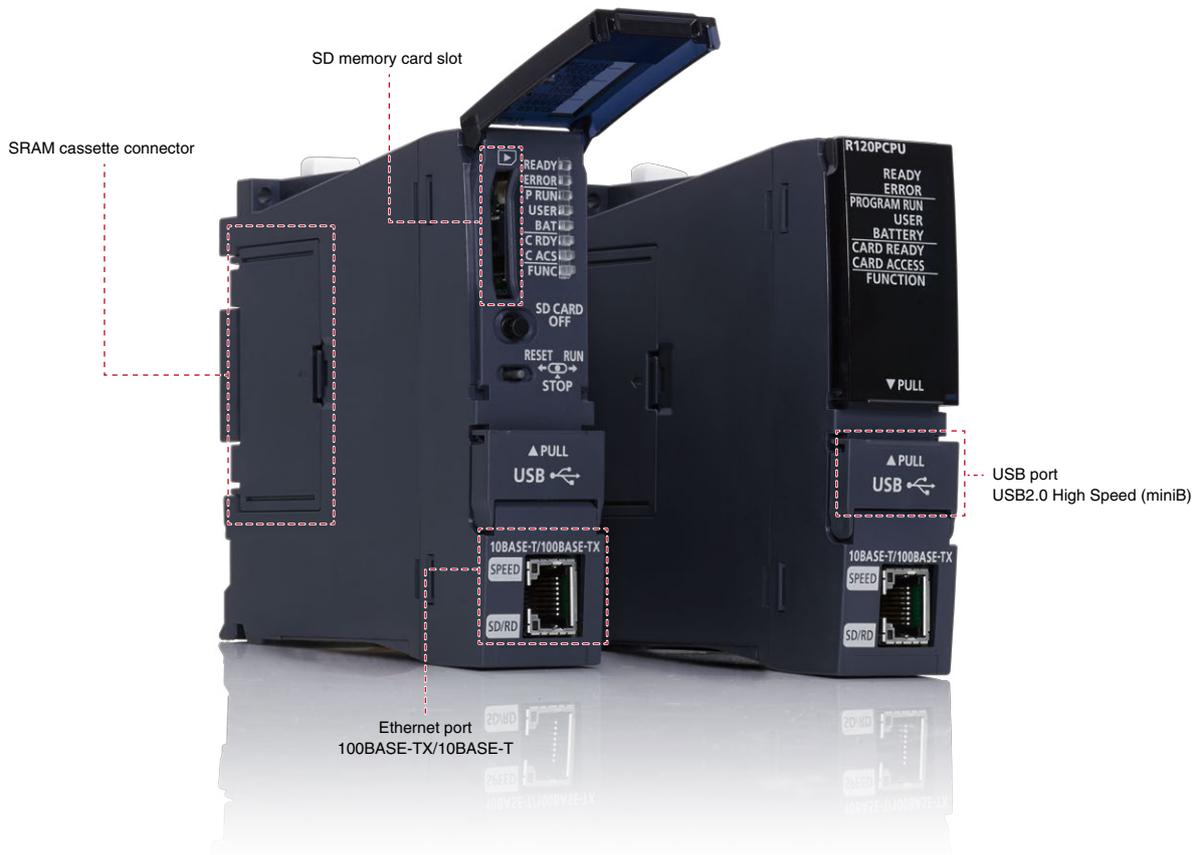
The Process CPU module is part of the application-specific range in the MELSEC iQ-R Series and has four CPUs available with memory sizes from 80K to 1200K steps. Designed specifically for medium- to large-scale process control systems requiring high-speed performance coupled with the handling of large PID loops. General control is possible with these modules, however, this range of CPUs also enables the hot-swapping of I/O modules, which adds further reliability to the control system.
