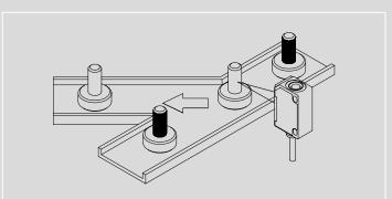
Rejection of uncoated parts
