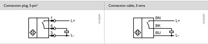
$<sup>^{\</sup>rm 4}$  Plug M12x1 3-pin is compatible with M12x1 4- or 5-pin sockets
