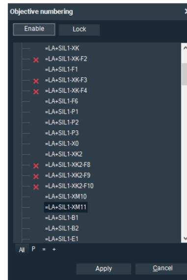
If these components are not to be shown as =LA-XK-..., then go to the settings and, under "Symbol Component box", clear the "Standard symbols" check box and confirm this, and then enable and confirm it later.
